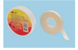
Scotch® 27 glass cloth electrical tape is a woven glass cloth tape designed to operate in applications requiring high mechanical strength and resistance to high temperatures. The glass cloth is specially treated and prepared to providecorrosion free protection. The glass will not shrink, rot or burn and has a high tensile strength. The adhesive is a rubber pressure-sensitive thermosetting system. The tape is designed for continuous use at class "B" (130°C) temperature.
