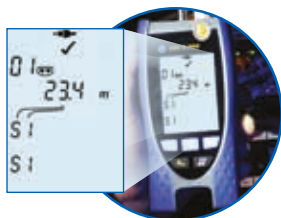
Test câblage coaxial
