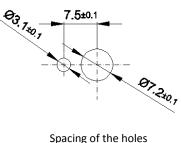
Spacing of the holes in the front panel
