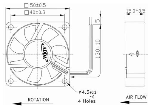
LEAD WIRES: UL 1007, AWG26, L = 130 +/- 10 mm Red = positive; Black = negative.
