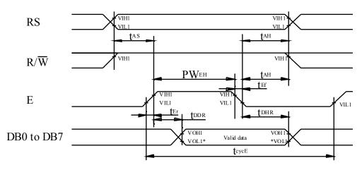
NOTE: \*VOL1 is assumed to be 0.8V at 2 MHZ operation.
