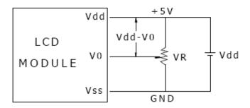
Vdd-V0: LCD Driving Voltage
