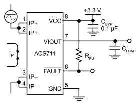
Application 1. The ACS711 outputs an analog signal,  $V_{IOUT}$ , that varies linearly with the bi-directional AC or DC primary current,  $I_P$ , within the range specified. The FAULT pin trips when  $I_P$  reaches ±100% of its full-scale current.
