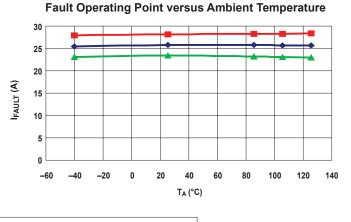
— Typical Maximum Limit 🛶 Mean 🛛 📥 Typical Minimum Limit
