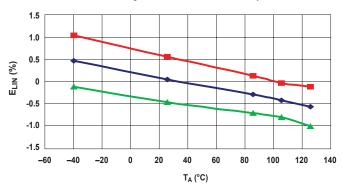
Total Output Error versus Ambient Temperature
