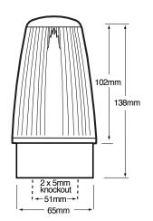
The X125 Series utilises a discharge capacitor and converter circuit to ignite xenon gas inside a tube, resulting in a brilliant flash of light. Xenon gas ignites virtually instantaneously so maximum brightness is
