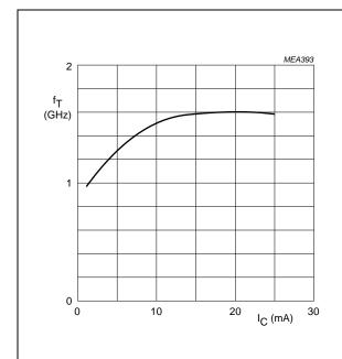
$V_{CE} = 5 \text{ V}; f = 500 \text{ MHz}; T_j = 25 \,^{\circ}\text{C}.$
