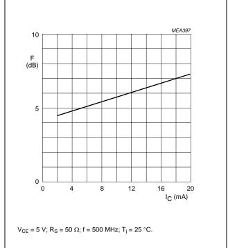
Fig.5 Minimum noise figure as a function of collector current.
