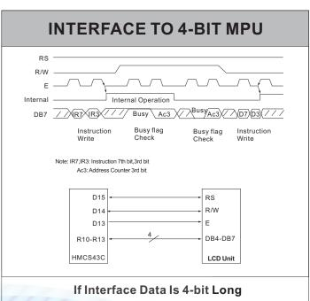
Data transfer is accomplished through 4 bus lines from DB4 to DB7. (while the rest of 4 bus lines from DB0 to DB3 are not used.)
