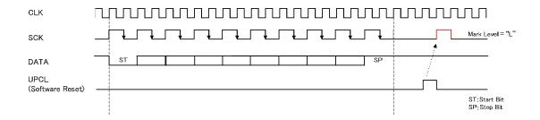
The connected slave device may consider this pulse on SCK line as a serial clock.
