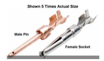
All pins and sockets can be easily wired using NEWPORT® thermocouple wire in either solid or stranded construction, 20 or 24 gage. Stranded wire is recommended so that electrical connections will have higher reliability. These precision Sub-D connectors are sold in sets of five, each package consisting of 5 male connector bodies and 5 female connector bodies. Sets are available in 9, 15, 25, 37 and 50-pin configurations.
