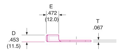
Max Electric Current: 4 AWG / 115 Amp
