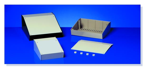
The 6000 range of small desk consoles are of a two piece construction. They incorporate 1mm thick, grey aluminium front panels which sit recessed into the top of the ABS bases and are held by four fixing screws running into integral brass inserts.
