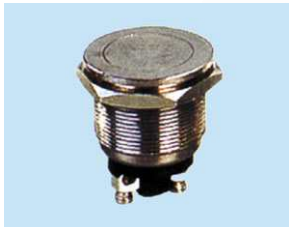
PS28B-2 OFF-(ON) 4 A 125 VAC; 2 A 250 VAC
