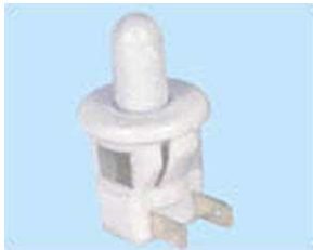
PS19B OFF-(ON) PS19C ON-(OFF) 5 A 125 VAC; 2.5 A 250 VAC
