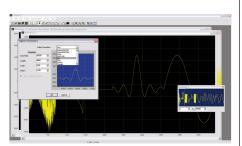
Use waveform editing software to easily generate, edit, and download custom arbitrary waveforms. Generate waveforms by importing a text file, or define via freehand, point draw, or waveform math. Waveforms can also be loaded from the generator for documentation purposes.
