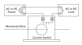
NOTE: The above diagram is for Normally Open (N.O.) models.
