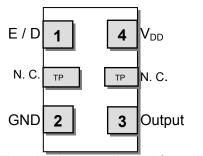
Terminations as viewed from the Top NOTE: XPRESSO HCMOS XOs are designed to fit on Industry Standard, 4 pad layouts
