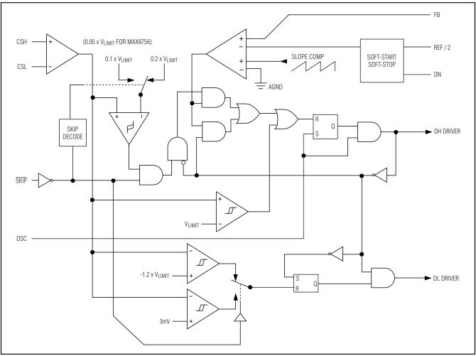
Figure 3. PWM-Controller Functional Diagram
