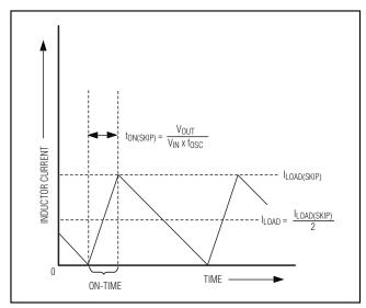
Figure 4. Pulse-Skipping/Discontinuous Crossover Point
