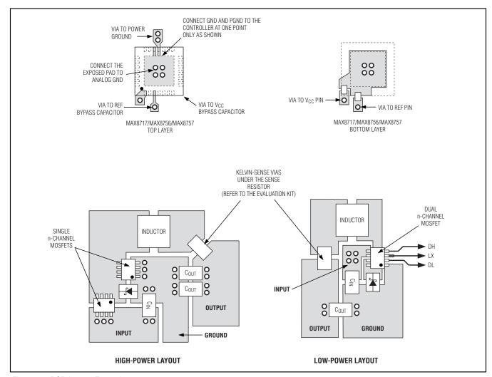
Figure 10. PCB Layout Example
