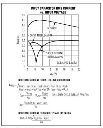
Figure 9. Input RMS Current
