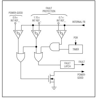
Figure 7. Power-Good and Fault Protection
