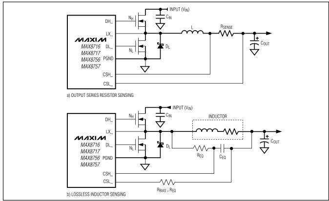
Figure 8. Current-Sense Configurations
