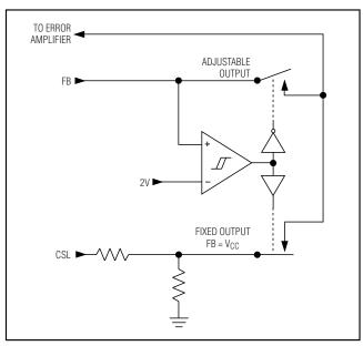
Figure 5. Dual Mode Feedback Decoder
