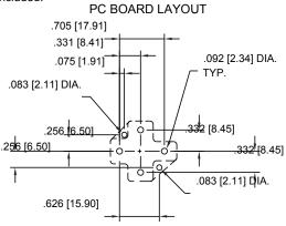
DZ85AB-5-PCB 5 Pin PCB Socket for 40 & 60 Amp Relays - Pins are Included.
