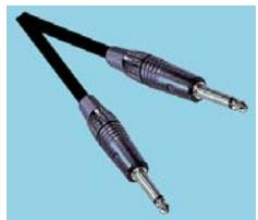
A range of excellent value loudspeaker leads fitted with Neutrik 2-Pole, 1/4" (6.35mm) Mono Jack plugs with rugged black bodies and featuring high quality, highly flexible cable (2x 1.5mm<sup>2</sup> conductors). Suitable for connecting most amplifier and powered mixers to speaker cabinets often used in disco, music and the PA industry.
