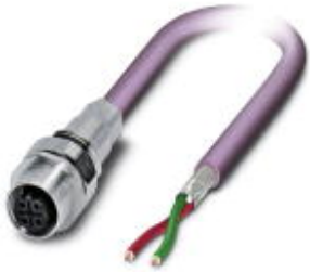
Bus system flush-type socket, PROFIBUS, 2-pos., M12, shielded, B-coded, front/screw mounting with M16 thread, with 5 m bus cable, 2 x 0.25 mm 2
