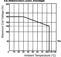
The maximum coil voltage refers to the maximum value in a varying range of operating power voltage, not a continuous voltage.
