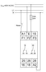
Range 300V, supply voltage 24V AC/DC and fault latch
