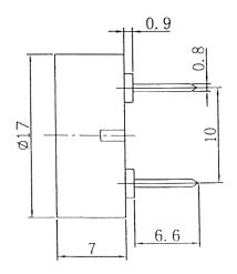
Dimensions: Millimetres Tolerance: ±0.3mm
