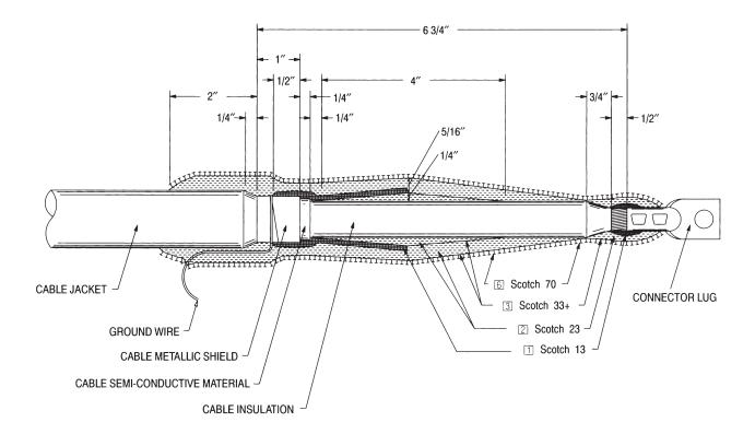
4. Allow the termination to air-dry in the upright position before applying the voltage.
