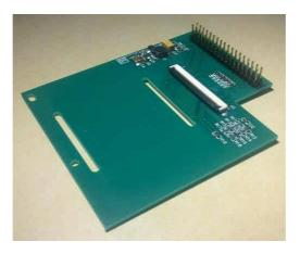
Figure 1. LCD connector expansion board for EM-AT91SAM3U
