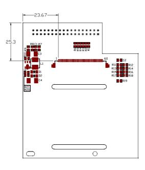
Figure 2. LCD connector Location (Bottom)
