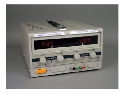
The **digimess**<sup>®</sup> SM series is a range of general purpose switch mode power supply units featuring high output currents and voltages. All models can operate in either constant voltage or constant current modes and feature large red LED displays for ease of viewing. The switch mode design results in small and light weight units compared to their linear equivalents. All units are supplied with mains leads and operating manuals.
