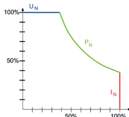
Units as from 1kW output power are equipped with a flexible autoranging output stage which provides a higher output voltage at lower output current, or a higher output current at lower output voltage, always limited to the max. nominal output power. See figure to the left.
