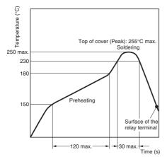
**Note:** Temperatures are given for the surface of the terminal.
