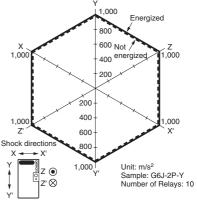
Conditions: Shock is applied in  $\pm X, \pm Y$ , and  $\pm Z$  directions three times each with and without energizing the Relays to check the number of contact malfunctions.
