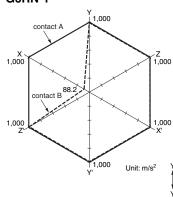
Sample: G6RN-1 24 VDC Number of Relays: 5 pcs Test conditions: The value at which malfunction occurred was measured after applying shock to the test piece 3 times each in 6 directions along 3 axes. Standard value: 100m/s² at contact A, 50m/s² at contact B
