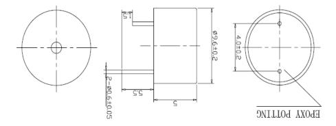
Dimensions Unit: mm Tolerance: ±0.5mm
