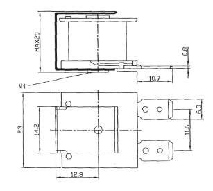
Dimensions: Millimetres Tolerance: ±0.5mm
