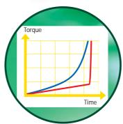
The red line indicates the steep increase in torque with hard applications, e.g. in metal.
