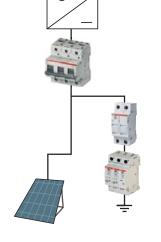
**OVR Surge Protective Device protection** E 90 PV fuse-disconnectors can be installed in field enclosure as back-up protection of Surge Protective Device.
