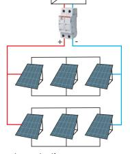
Inverter protection In small photovoltaic plants, inverter protection against overload and short-circuit is possible by means of E 90 PV.
