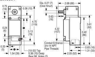
• Can accommodate both U.S., 1.16 (29.4) x 2.34 (59.5) and DIN, 1.18 (30) x 3.26 (60), mounting dimensions.
