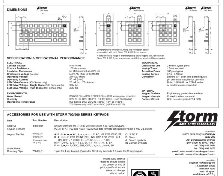
All dimensions in millimetres (mm) Full product specifications are available on request from your local Storm supplier. Storm keypads incorporate key switch technology protected by International Patents.
