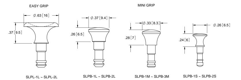
NOTES: 1. PLUNGER MATERIAL: NYLON 6, (RMS-120). 2. GROMMET MATERIAL: POLYCARBONATE, (RMS-72). 3. COLOR: BLACK OR WHITE; ADD SUFFIX "-B" OR "-W" TO PART NO.
