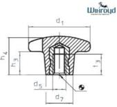
Material Grip: Duroplast FS 31 DIN 7708, black Threaded bush: steel, galvanised. 7006.W220 - brass. Temperature range: max 110° C.
