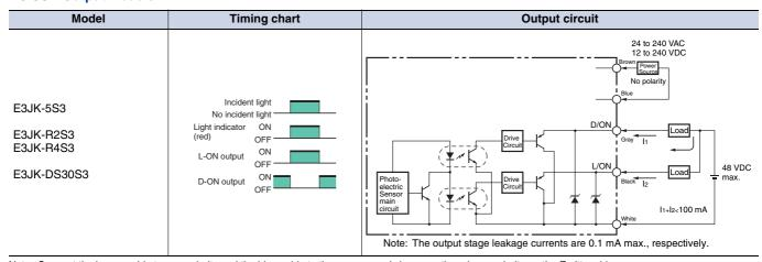
Note: Connect the brown cable to any polarity and the blue cable to the power supply because there is no polarity on the Emitter side.
