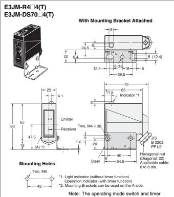
mode switch are located inside the cover.
