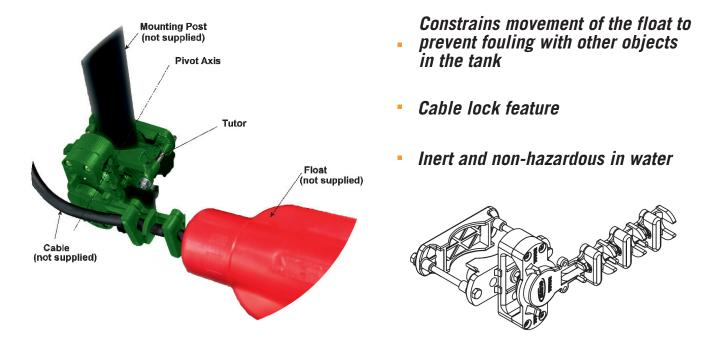
Equipped with a special bracket, the **Tutor** system can be easily fixed directly on pumps, or wall fixed, or on pipework for steering the floating switch in narrow or confined spaces to avoid the accidental fouling of other pipes, cables, walls and other obstacles.
