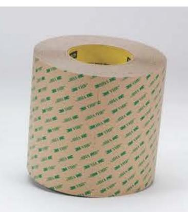
3M<sup>™</sup> VHB<sup>™</sup> Adhesive Transfer Tape F9460PC case is a 6.2 mil, 3M<sup>™</sup> High Performance Acrylic Adhesive 100MP tape on a 4.2 mil, Tan 58# Polycoated Kraft Paper (PCK) liner.
