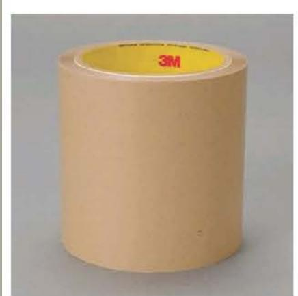
3M™ Double Coated Tape 9500PC is a 5.6 mil 350 high performance acrylic adhesive double coat with polyester carrier on a 4.5 mil 61.5 lb polycoated kraft paper liner.
