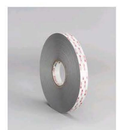
3M™ VHB™ Tape 4941 is a conformable, double-sided, pressure-sensitive, closed-cell acrylic foam tape with a paper liner, 45 mil thick.
