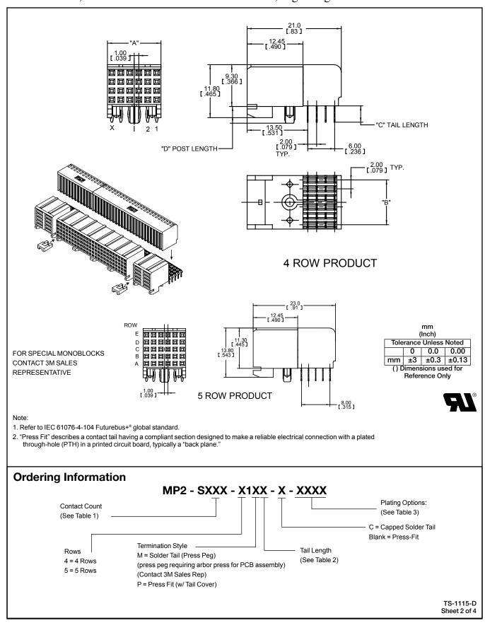
2 mm 4/5-Row, Solder Tail or Press-Fit With Tail Cover, Right Angle
