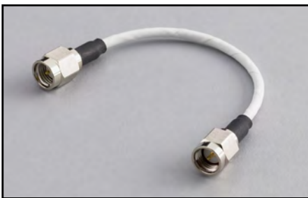
CA-451A: 10.8cm (4.25 in) RG188 coax cable terminated with an SMA male plug on each, 50Ω impedance.
