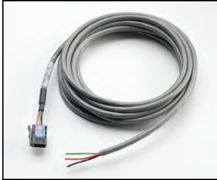
Model 2290-INT-CABLE: Safety interlock cable, 3.05m (10 ft). 3-conductor cable with 3-pin connector on one end and unterminated wires on the other end.
