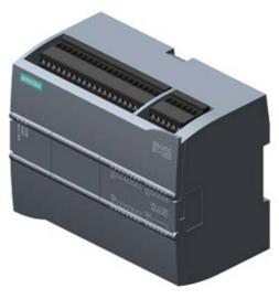
SIMATIC S7-1200, CPU 1215C, COMPACT CPU, AC/DC/RELAY, 2 PROFINET PORT, ONBOARD I/O: 14 DI 24V DC; 10 DO RELAY 2A, 2 AI 0-10V DC, 2 AO 0-20MA DC, POWER SUPPLY: AC 85 -264 V AC AT 47 - 63 HZ, PROGRAM/DATA MEMORY: 100 KB
