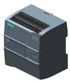
SIMATIC S7-1200, CPU 1211C, COMPACT CPU, AC/DC/RELAY, ONBOARD I/O: 6 DI 24V DC; 4 DO RELAY 2A; 2 AI 0 - 10V DC, POWER SUPPLY: AC 85 - 264 V AC AT 47 - 63 HZ, PROGRAM/DATA MEMORY: 30 KB
