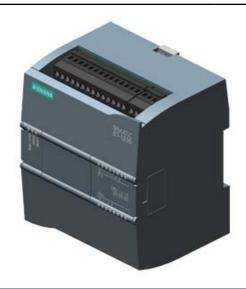
SIMATIC S7-1200, CPU 1211C, COMPACT CPU, DC/DC/DC, ONBOARD I/O: 6 DI 24V DC; 4 DO 24 V DC; 2 AI 0 - 10V DC, POWER SUPPLY: DC 20.4 - 28.8 V DC, PROGRAM/DATA
