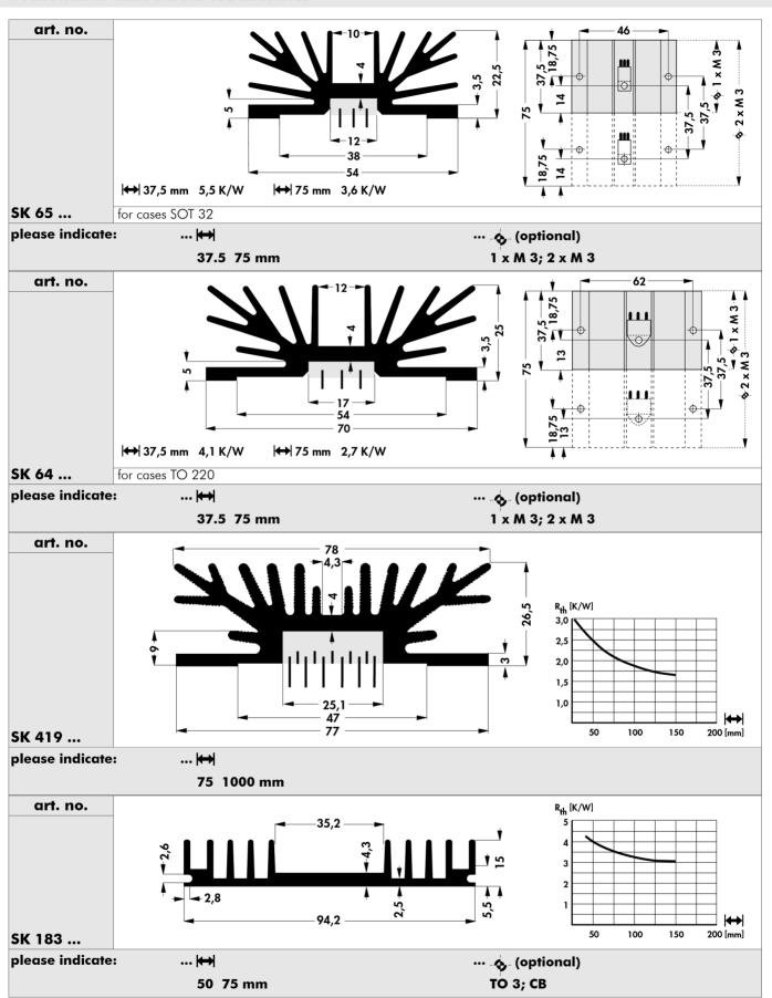
Mounting for TO 3 angle Order example Attachable heatsinks for TO-cases Heatsinks for DC/DC converter
